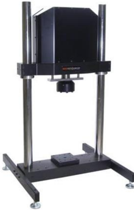
Figure 3.7. 800 series UTM fatigue test machine (Adopted from www.testresources.net )
